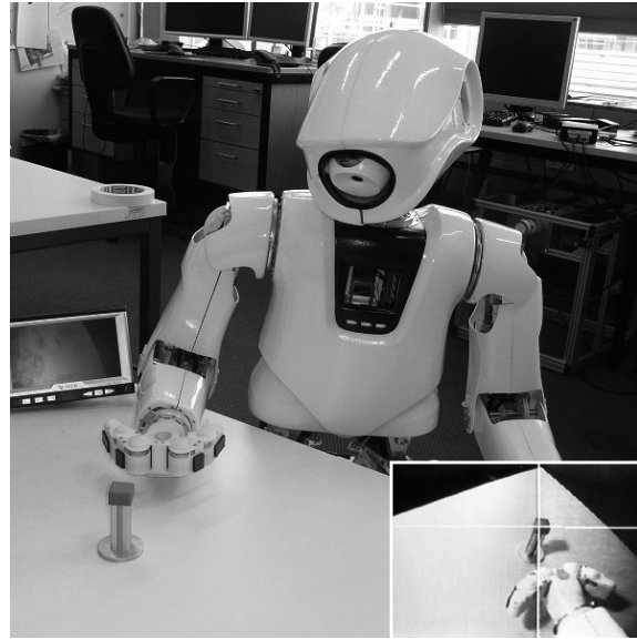
Figure 8: Myon sitting at a table and performing a gripping task using hand-eye coordination. In the lower right the image of the robot's camera is shown. The recognized object is shown using a cross hair.
