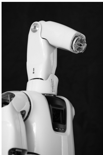
Figure 1: All body parts of the robot MYON can be detached and reattached during runtime. Here, the head has been replaced by the robot's left arm.
